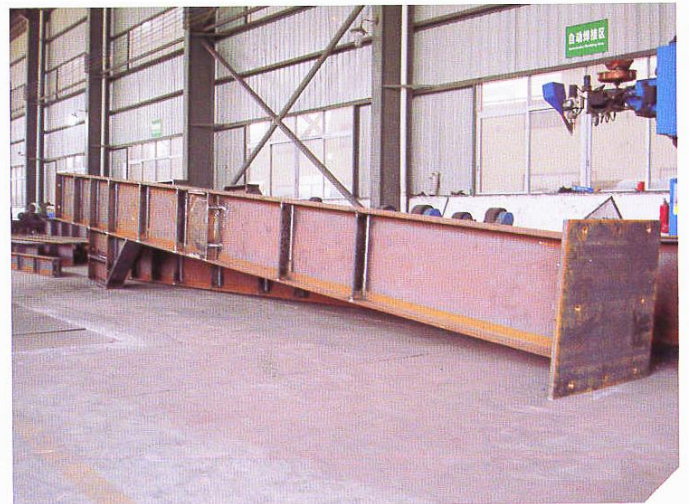
伸缩臂/Telescopic Boom 规格/Specification: 7500mmX760mmX700mm
