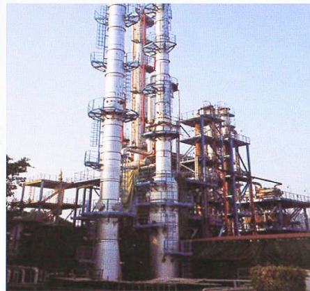
抽提蒸馏塔(T-702, 图左)和溶剂回收塔(T-703, 图右)现场安装图 Extractive Distillation Column (T-702, the left column) and Solvent-recovery Column (T-703, the right column) are completely installed.
