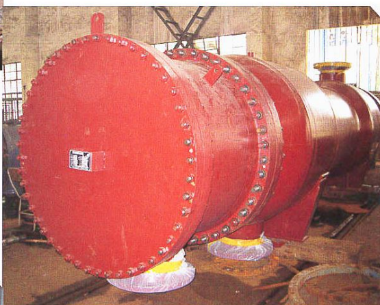
浓硫酸罐/Concentrated Sulfuric Acid Tank 规格/Specification: OD2200mmX12mmX5800mm
