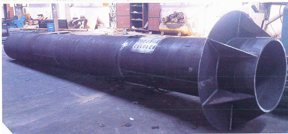
平口管 (带1个铁环, 6件三角板) / Plain end Pipes (with one ring plate and six triangle steel plates)
