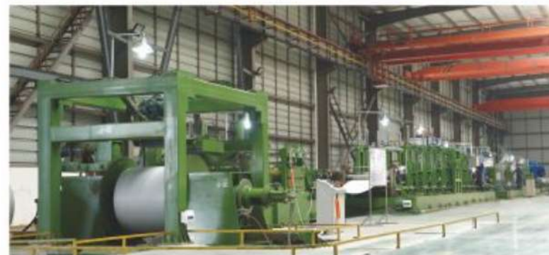
130型号机组生产线 (最大外径426mm) The 130 type unit production line (The maximum outer diameter is 426mm)
