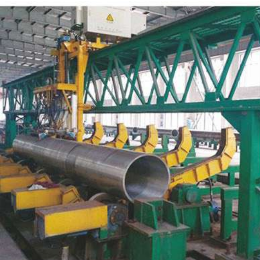
< Magnetic flux leakage & ultrasonic testing line
